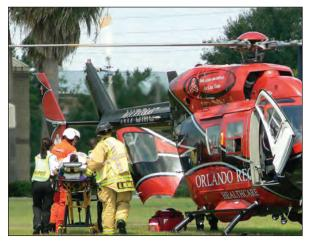
Fig. 27-10: Tail rotors are dangerous. Approach only if given permission by the pilot and only from the front or side so the pilot sees you. *Courtesy of Ted Crites*.
