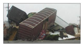
Fig. 29-4: Unusual placement or conditions and leaking containers are indications of the presence of hazardous materials. Courtesy of Capt. Tony Duran, Los Angeles County Fire Department.
